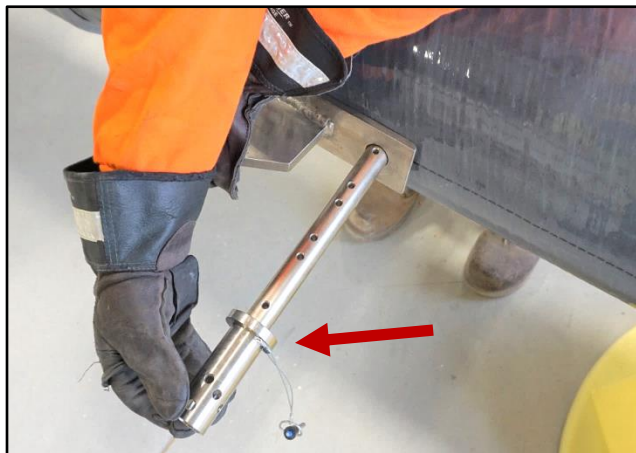
Figure 17: Install the retention collar onto the jacking bar with the flanged side toward the jacking plate.
