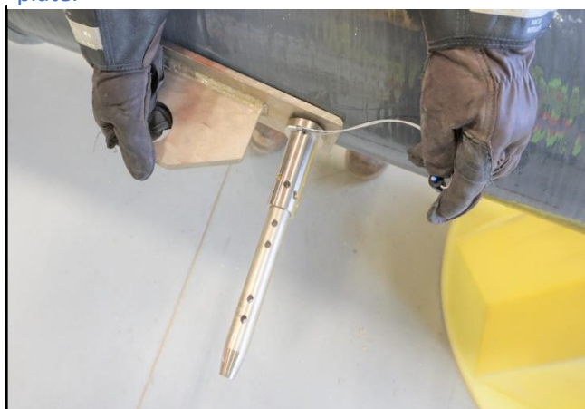
Figure 18: Rotate the retention pin to find the most suitable hole to keep the plate tight against the module wall.
