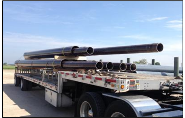
Figure 2 - Partially Pre-assembled - two or more modules are assembled, with remaining modules nested inside the partially assembled modules.
