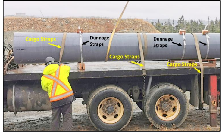
Figure 6: Highlighting the difference between cargo strapping and dunnage strapping.
