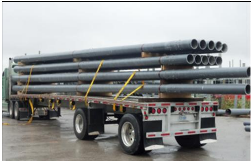
Figure 3 - Fully Assembled - The pole is fully assembled at the factory with slip joints secured. Top caps, base plates and hole plugs may require field installation prior to installation.
