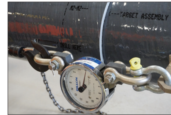
Figure 14: Completed Slip Joint Assembled to 4,000 lb. [1,814 kg] of Force
