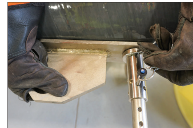
Figure 10c: Inserting the Quick Release Pin With the Retention Collar Tight to the Jacking Plate
