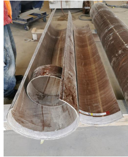
Figure 7: Primary shield and cover strip prepared at factory.
